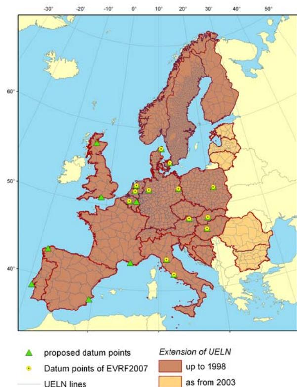
**Figure 2 Proposed and finally used datum points**
